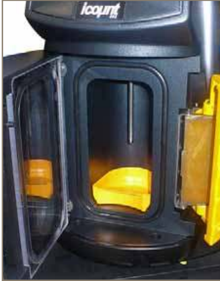
Fig 4. The IBS2 oil sampling probe automatically lowers into the bottle once the test begins.
