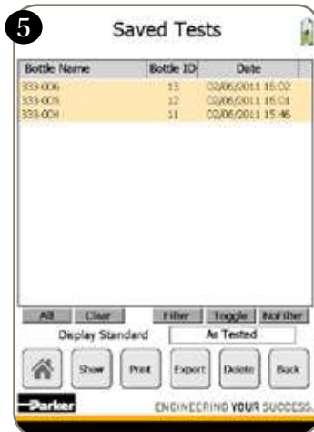
Export results: Highlight the test result(s) you would like to export using the stylus.
