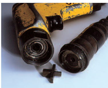
Damaged pneumatic tooling
